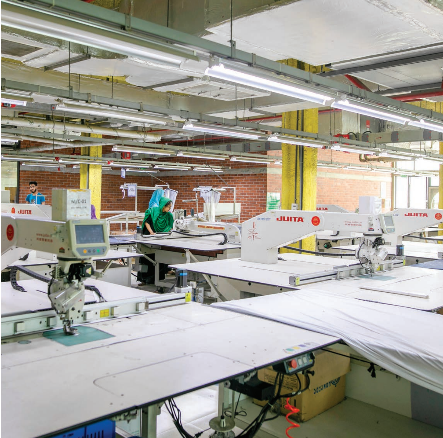
These energy-efficient, automated template sewing machines at the Fakir Eco Knitwears factory near Bangladesh's capital help workers reduce waste.
